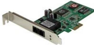
The PEX1000MMSC2 PCIe Gigabit Fiber Network Card lets you connect a desktop PC directly to a fiber optic network, by adding a multimode SC fiber port to your computer or server through an available PCI Express slot.
