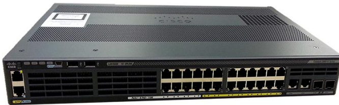
Figure 4. Fanless Quiet Cool 24-Port PoE Switch
